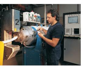
The silicone compounds then undergo the extrusion process, in which the tool (die) creates the actual contour. Vulcanisation follows in a heating section without external pressure (pressureless vulcanisation) with platinum catalyst for addition curing or with peroxide curing.
