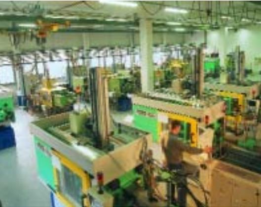
The automotive industry is a major sector for LSR applications: here BIW produces connector seals for cable sets and vehicle networks in line with the automotive and OEM specifications such as SAEJ-200xxx, DBLxxx, VW 2.8.1xxx or Bosch N2580-x.
